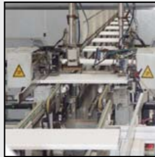
throughfeed NC machines for boring and boring/dowel inserting
